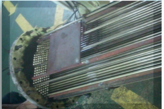
Boiler and Heat Exchanger retubing
