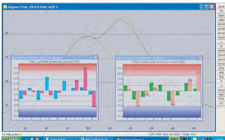
The **EDS** helps to reduce the engines' operating cost. Cylinder - to Cylinder load balancing and correct fuel injection settings will optimize engine performance, minimize specific fuel oil consumption and reduce Emissions.
