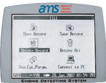
The **EDS** is designed as a stand alone unit. The long battery life, the 320 x 240 pixels screen allows operation without a PC. The large non-volatile memory stores 60 measurement records, up to 20 cylinders each. The engine library can keep 30 engine data files.
