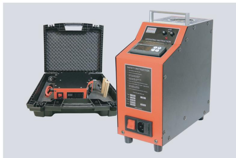
As the calibrators are portable, there is no need for ship instruments to be removed from their equipment boards, thereby reducing the risk for measuring errors and equipment damage.
