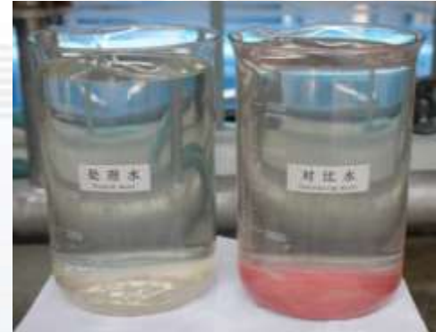
Comparison of water samples before and after hydraulic spin separation
